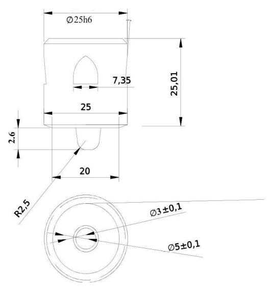
3. Tungsten Carbide tool with pin length of 2.5 mm required as per the diagram - 5 nos.
