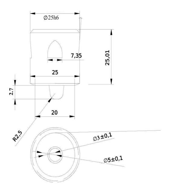
2. Tungsten Carbide tool with pin length of 2.6 mm required as per the diagram - 5 nos.
