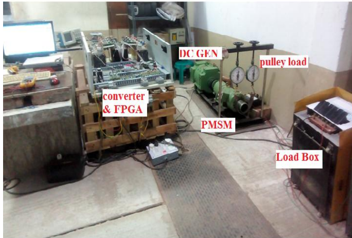
5 kW PMSM- Complete test set-up
