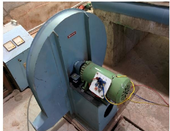
Real life testing of 0.75hp BLDC motor coupled with blower-fan load .
